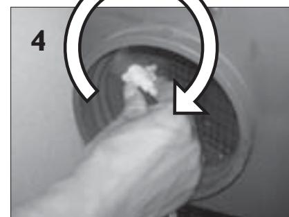
Turn the connector 90° clockwise until it is locked in place.
